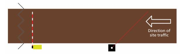
Position the SOSEC barrier at least 9m from the protected asset, switch it on and complete the setup procedure as laid out within this document in <u>Setup and first use</u>. Then, for a site speed limit of 10mph, position the over height sensor at least 31m up the road. Using the cable reel, run the connection cable back to the barrier and connect the cable to the barrier using the socket on the outside of the cabinet, under the power switch.
